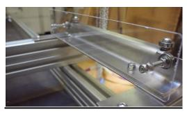
**3.** Sandblasted stainless steel joint for the handle.
