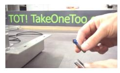
**2.2** Fix the router bit with sharp tip to the router.
