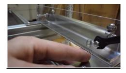
**7.10** Tight the inside nyloc nuts with 10 mm fork key. Plexiglass guard has to be locked tightly between the nyloc nuts.
