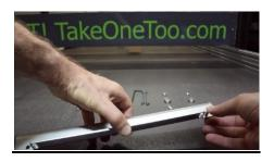
**4.3** Put the washer onto the screw.
