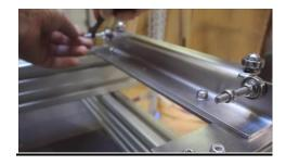
**7.8** Put the plexiglass guard onto M6x60 screws. Screws have to go through the holes in plexiglass guard.
