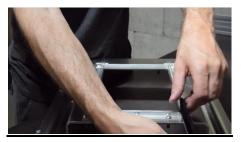
**5.3** Release the sealing brush. It has to hold tightly into the F aluminum slot.
