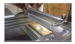
**7.7** Put the nyloc nuts M6 approx. 15mm from the end onto the both screws M6x60.
