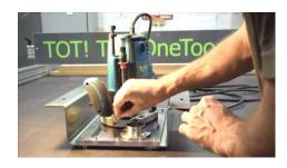
**2.7** Take out the router from TOT! cart and loose the screws from router's base.
