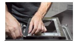
**5.2** Insert long sealing brush into the long F aluminum slot until is spring at the end of slot pushed. Then insert securing R clip back into the front holes of F aluminum slot. Release the sealing brush. It has to hold tightly into the F aluminum slot.
