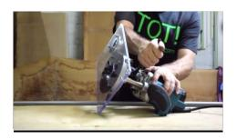
**3.5** The right depth of router bit in the router allows the router bit rotate freely into the center hole in the plexiglass base.
