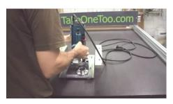
**2.4** Carefully set the router to the bottom position. Router bit's sharp tip has to be placed into the center of nesting hole. Lock the router in this position.
