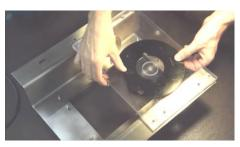
**2.10** Secure the router's base exact on the marked line on the plexiglass.
