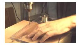
**2.13** Carefully break open the centering 40mm plexiglass wheel from the plexiglass base.
