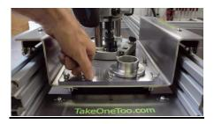
6.6 Put the vacuum cleaner hose adapter onto the stainless-steel flange. In case your vacuum cleaners' hose is 50 mm, cut the adapter at the end of 50 mm part. In case your 32 mm hose does not fit accurate into the adapter, use blue tape to tune the adapter diameter.
