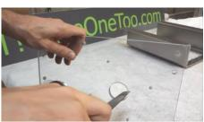
**2.16** Place the plexiglass plate on the bottom of the router.
