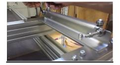
**7.5** Replace the screw M6x60 instead of M6x20.
