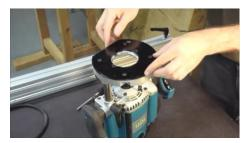
**2.9** Put the router's base exact on the marked line on the plexiglass.
