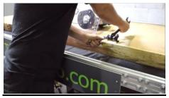
**3.4** Put the extended router bit into the router through the center hole in the plexiglass as deep as possible.
